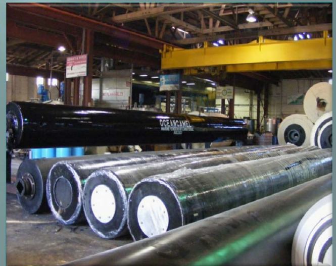
US COAST GUARD, MA STEEL CAMEL / URETHANE FLOTATION FOAM CORE
